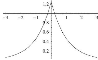
Figure 8.3 Filter function proposed by Castan et al. [Castan1990].
