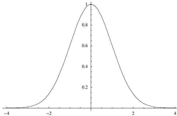
Figure 8.5 The Gaussian kernel ( $\sigma = 1$ ).
