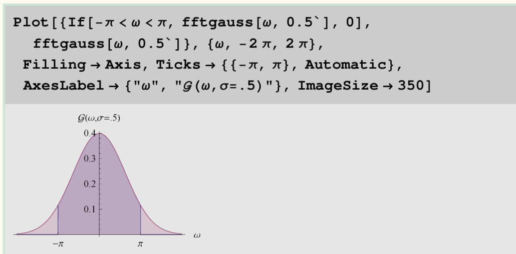
Figure 7.3 The definition of the leakage is the (unshaded) area under the curve outside the definition domain, relative to the total area under the curve. Here the definition is given for the 1D Gaussian kernel. Due to the separability of Gaussian kernels this definition is easily extended to higher dimensions.
