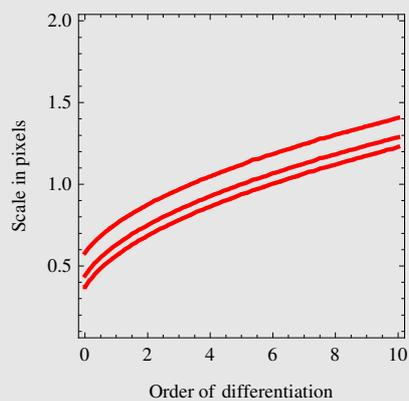
Figure 7.5 Relation between scale  $\sigma$  and the order of differentiation  $n$  for three fixed accuracies for a convolution with a Gaussian derivative function, implemented through the Fourier domain: upper graph: 1%, middle graph: 5%, lower graph: 10% accepted error.
