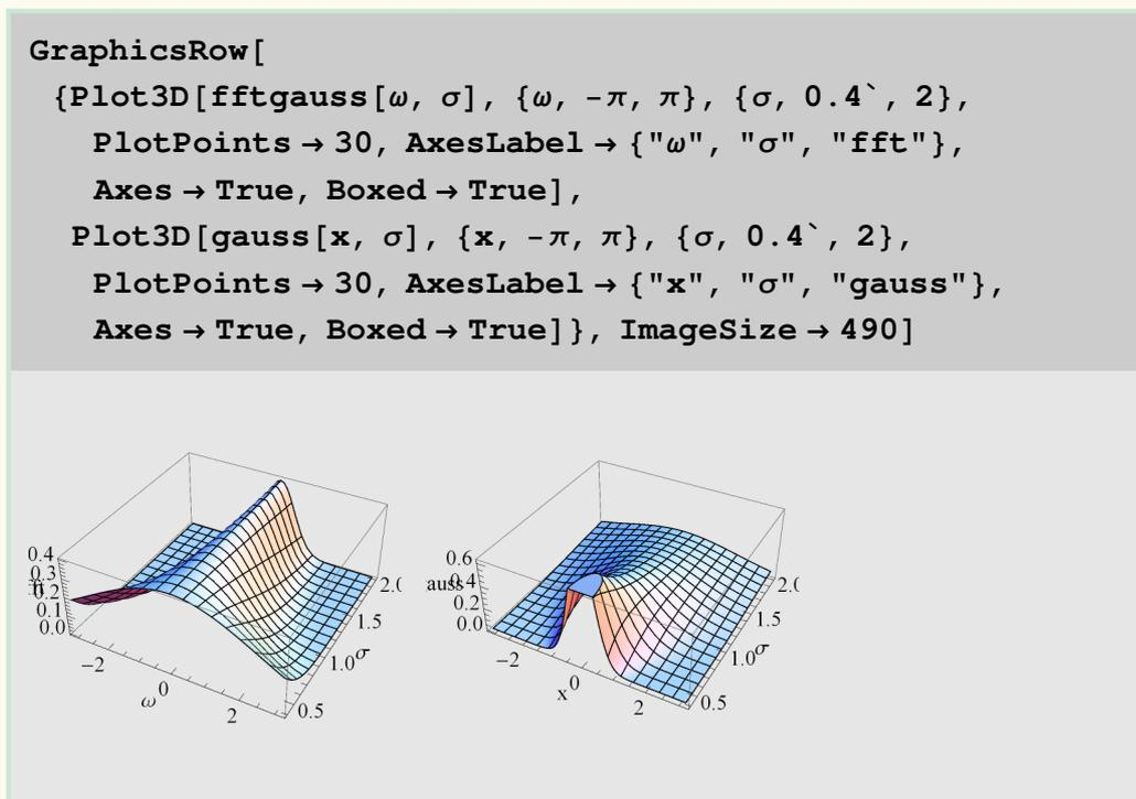
Figure 7.2 Left: The Fourier transform of the Gaussian kernel is defined for  $-\pi < \omega < \pi$ . The function repeats forever along the frequency axis over this domain. For decreasing scale  $\sigma$  in the spatial domain the Fourier transform gets wider in the spatial frequency domain. At some value of  $\sigma$  a significant leakage (aliasing) occurs. Right: The spatial Gaussian kernel as a function of scale.
