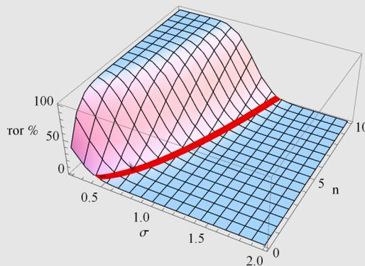
Figure 7.4 Relation between scale  $\sigma$ , order of differentiation  $n$ , and accepted error (in %) for a convolution with a Gaussian derivative function, implemented through the Fourier domain. The red line marks the 5% error.
