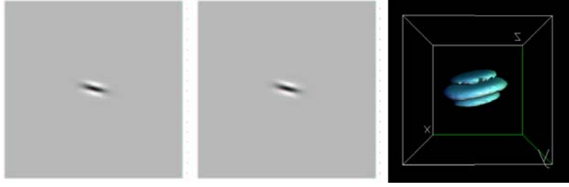
Figure 12. Density plots of through XOZ -plane and YOZ -plane of the 3D-equivalent (for details see Duits et al., 2004) of the 2D-wavelet obtained in the simple approach framework, see (20), a joint contour plot of iso-surfaces of this 3D-equivalent \psi at \psi(\mathbf{x}) = +0.02 and \psi(\mathbf{x}) = -0.02 , show that it is rather a surface patch detector than a line detector.
